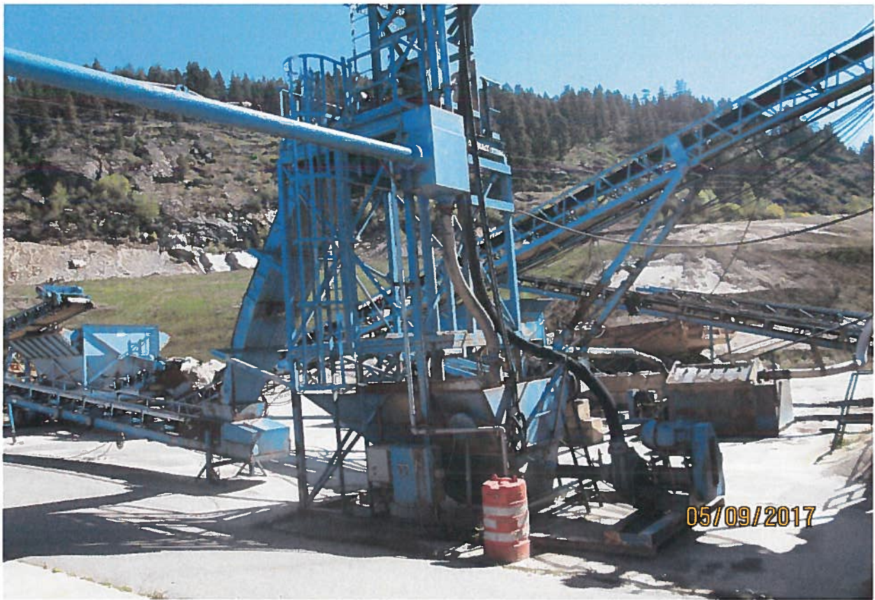
Water cleaning device that separates sand, mud, and other materials from water.
