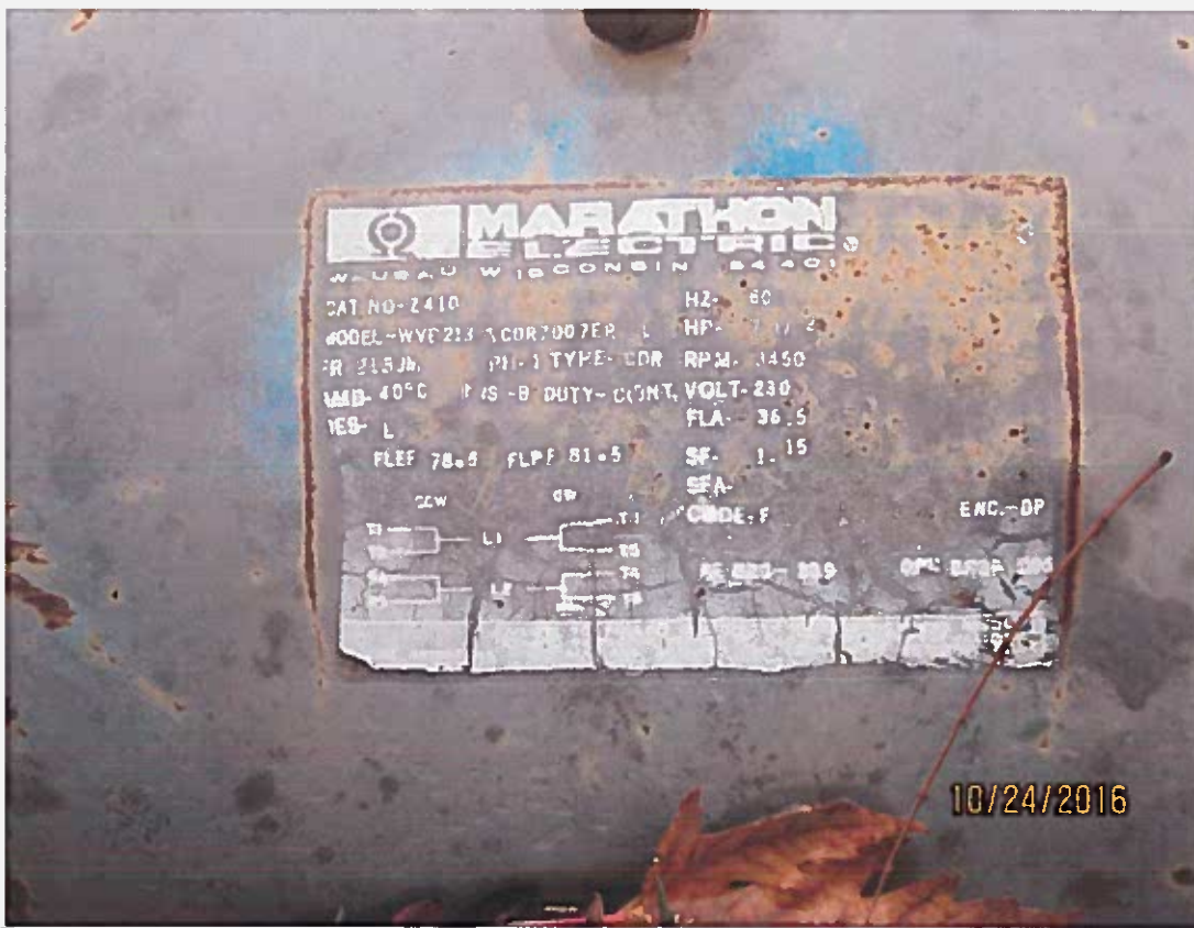
Marathon Electric motor. Serial # WVEZ13TCOR700ER
