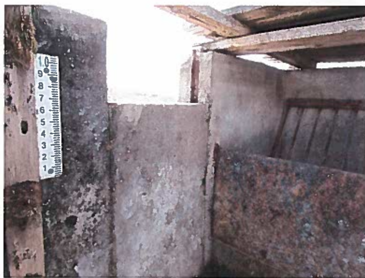
Pic of the staff gauge and plate. Kent Clegg says they never go over 4 inches of head.
