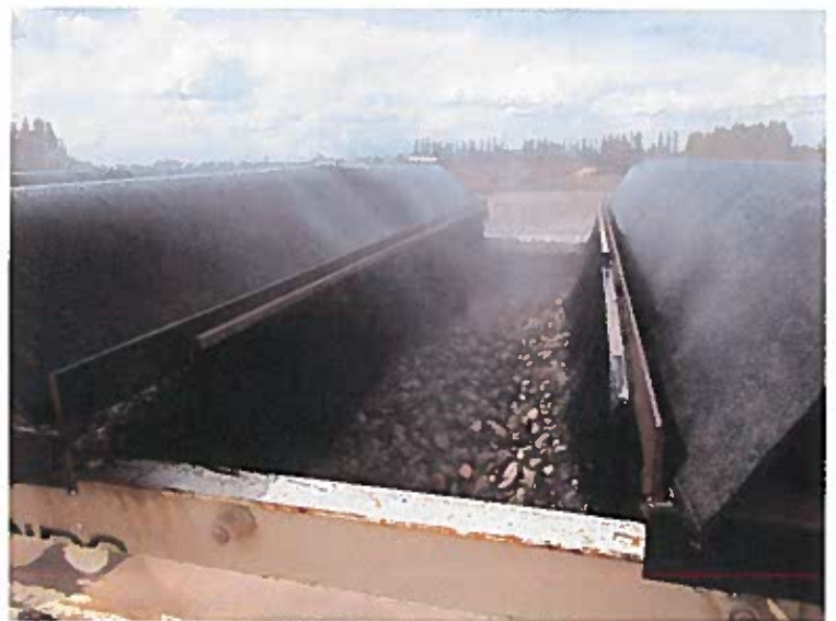
Close up of washing station, highlighting the shade covers and brushes to help reduce evaporative losses.
