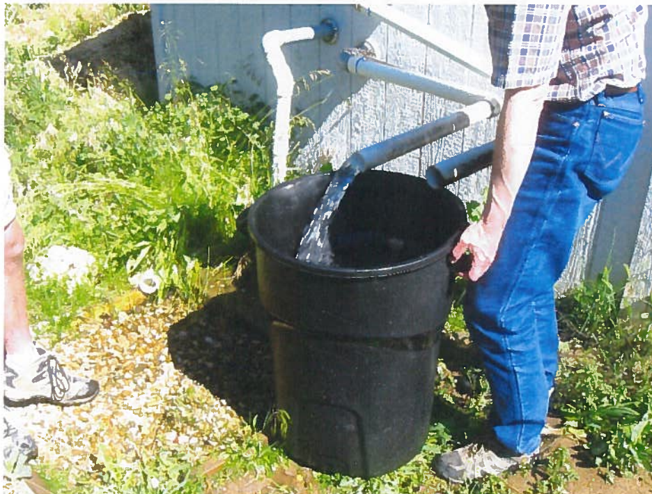
32-gallon trash can for volumetric flow measurement
