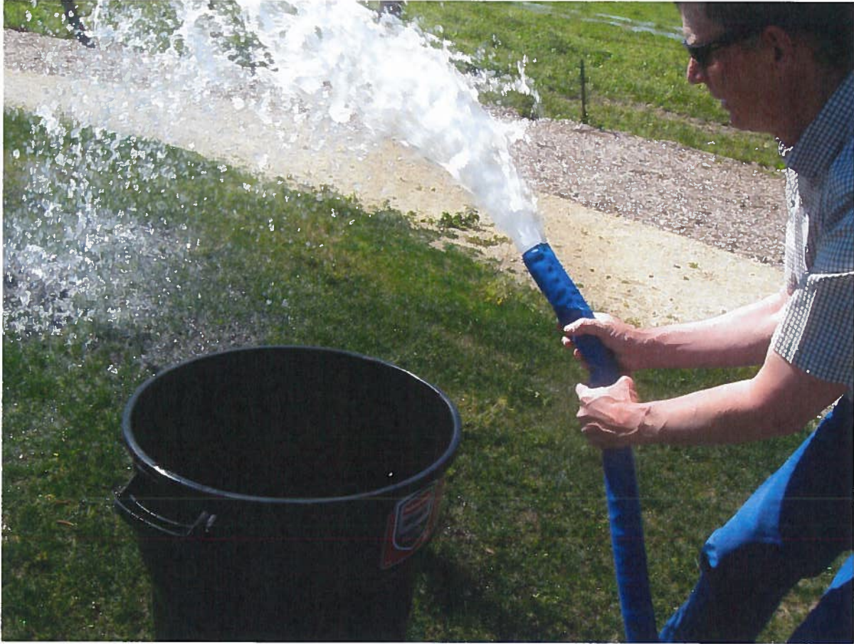
32-gallon trash can used for flow measurement.
