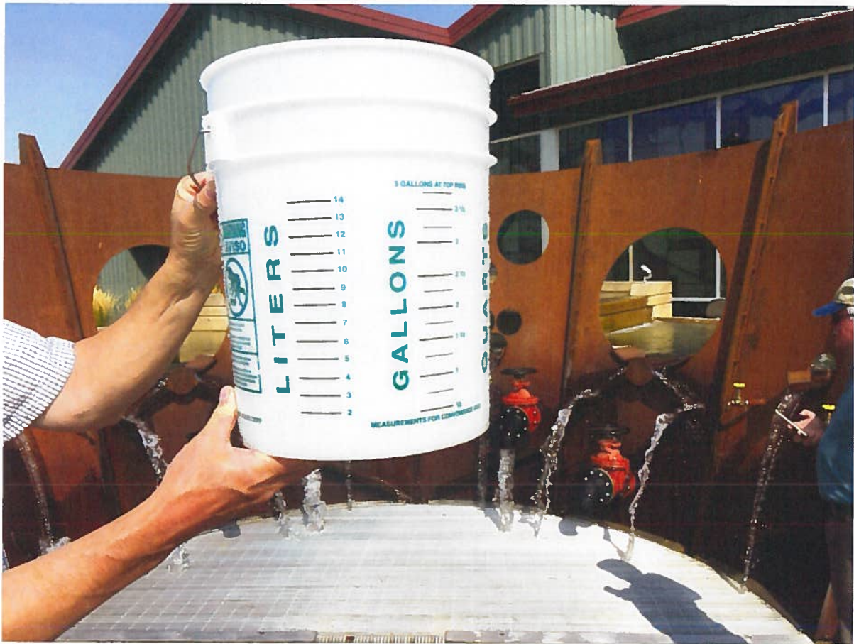
Calibrated 5-gallon bucket used for timed fill measurements
