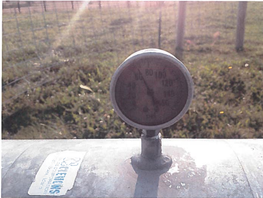
Figure 3 Pressure gauge at the well reading approximately 65 psi.
