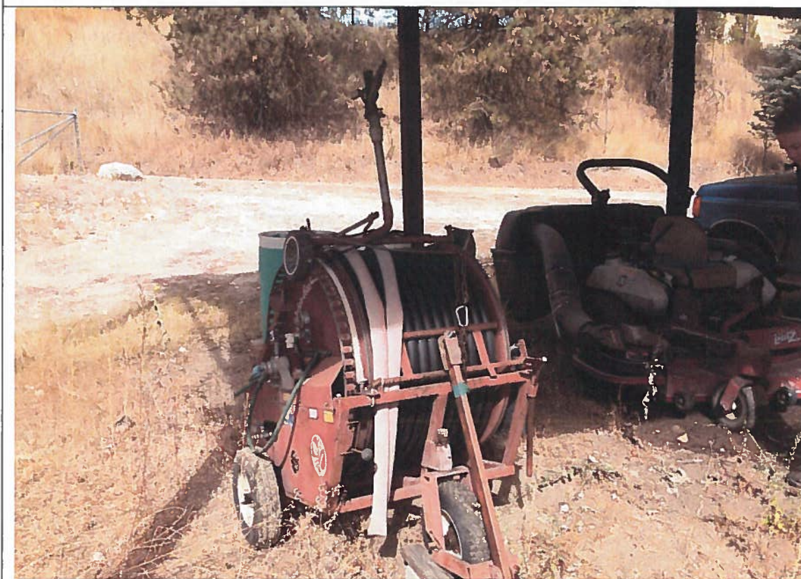
Roll out sprinkler used to deliver water to west portion of property
