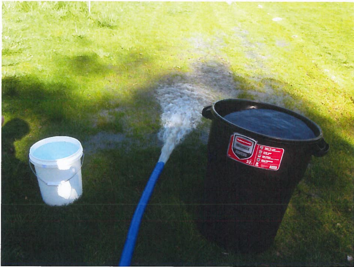
Temporary 2-inch hose, 5-gallon bucket, and 32-gallon trash can for volumetric flow measurement
