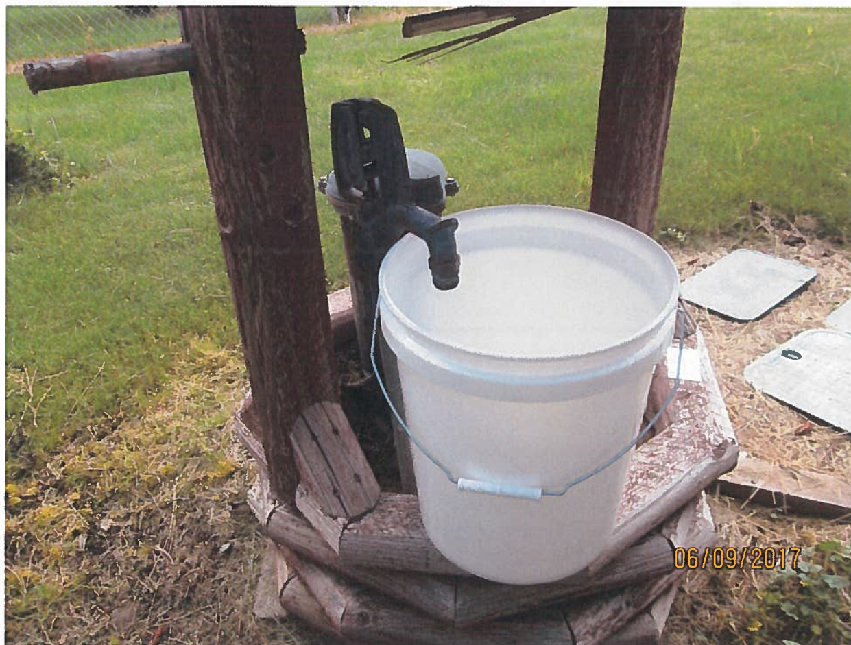
5 gallon bucket test performed in 11 seconds which is equal to 27 gpm or 0.06 cfs.
