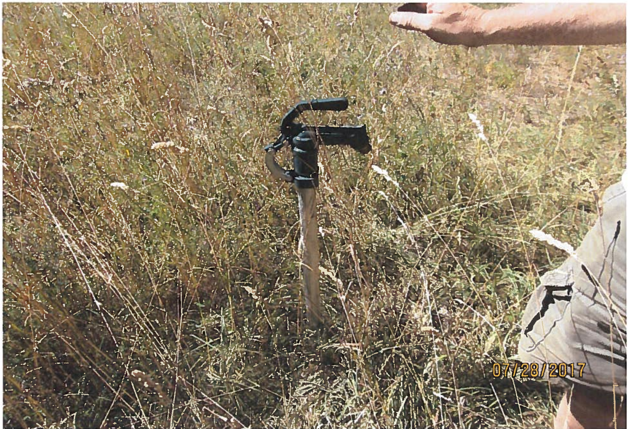
5 gallon bucket test performed filling in 11 seconds which is equal to 27 gpm or 0.06 cfs.
