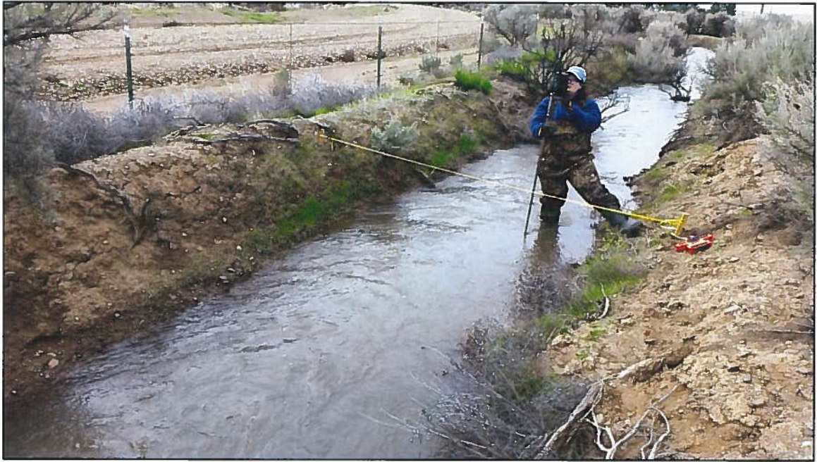
Figure 7: Measuring discharge at lower diversion.
