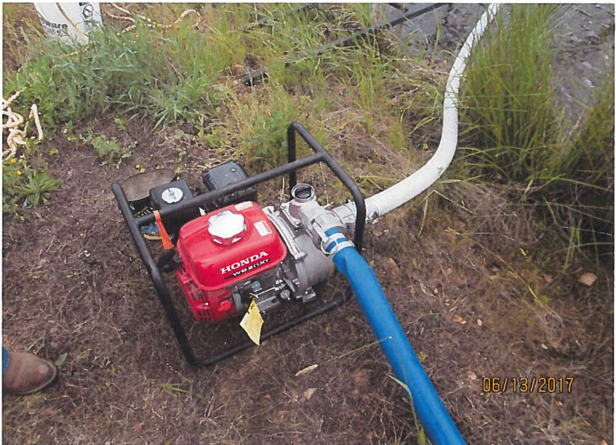
Honda pump capable of producing 164 gpm.
