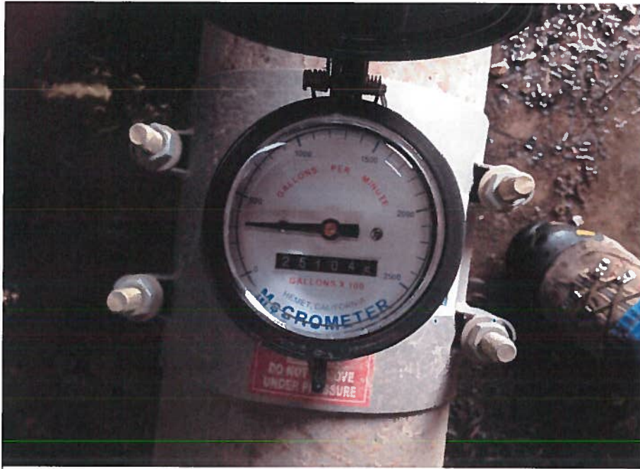
Figure 3 The propeller-type flow meter installed at the well. I used the flow meter to read the flow rate while the pump was running and the pipe was fully opened. This picture was taken when the pipe was partially closed.
