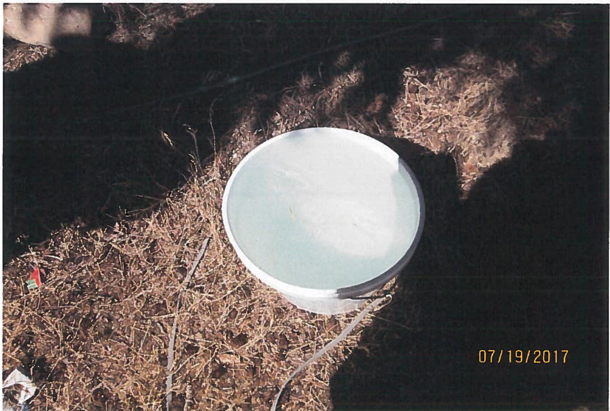
5 gallon bucket test performed in 40 seconds or 7.5 gpm or 0.02 cfs.
