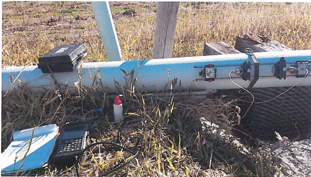
Picture 7. The setup used to measure the Lower Well.
