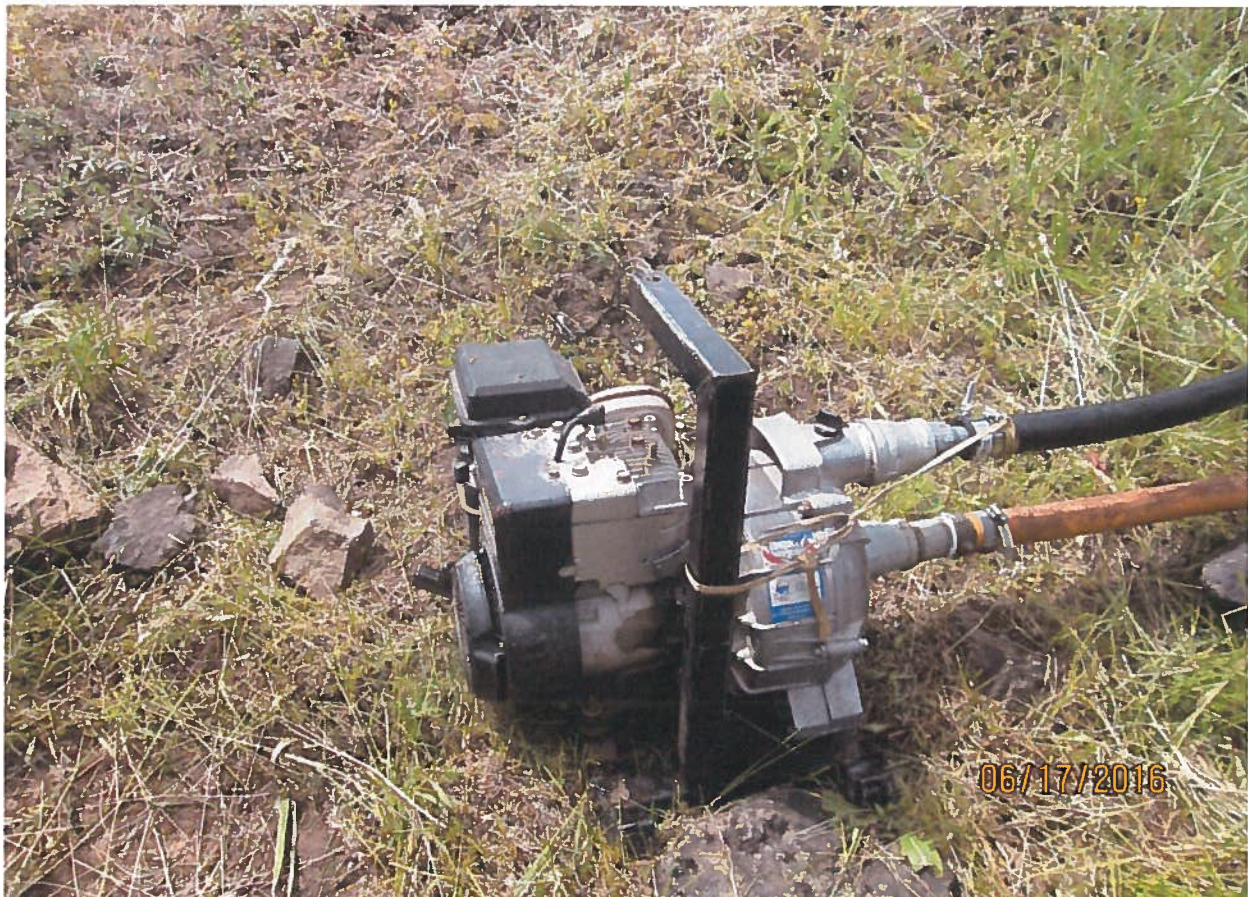
Pump 2. 2hp pump with diversion rate of 18 gpm.
