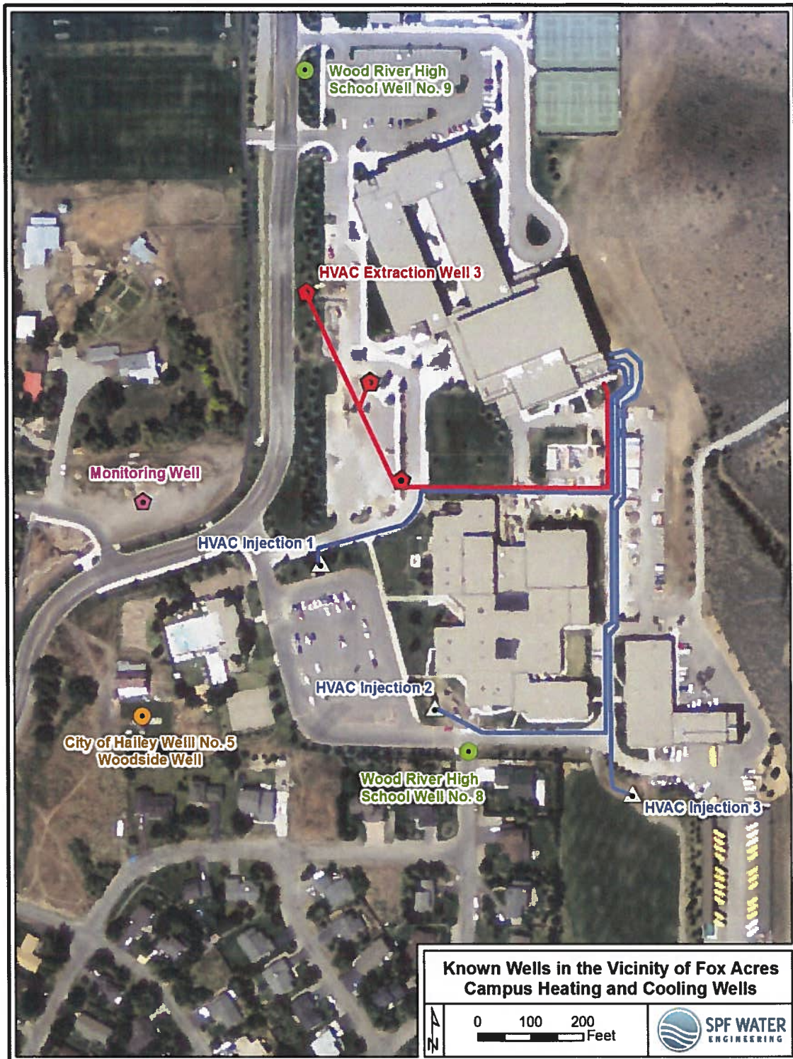
Figure 1. Fox Acres Campus Heating and Cooling Wells.
