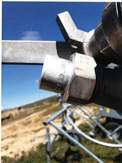
Figure 4 The Nelson 20 mm nozzle. Same on all reels.
