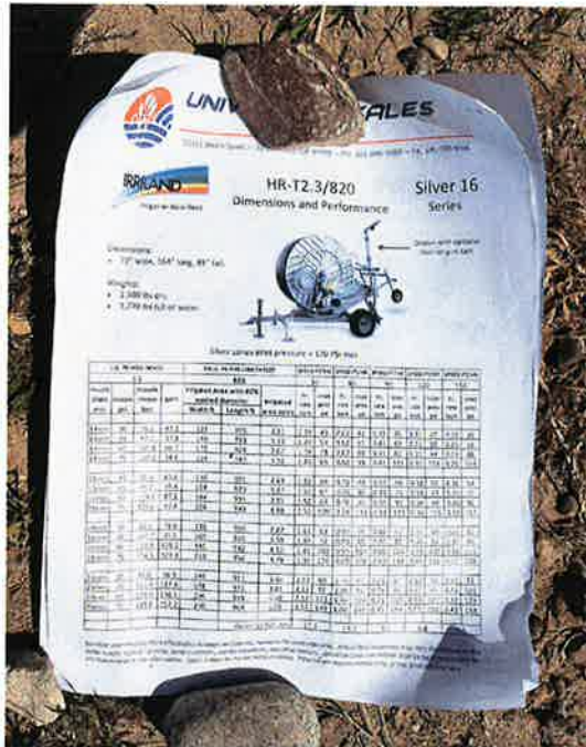
Figure 3 The performance sheet showing 136 gpm from the 20 mm nozzle at 60 psi.
