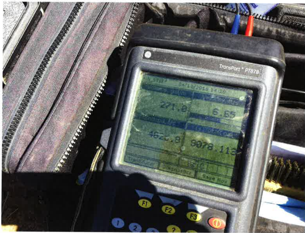
Portable ultrasonic flow meter readout
