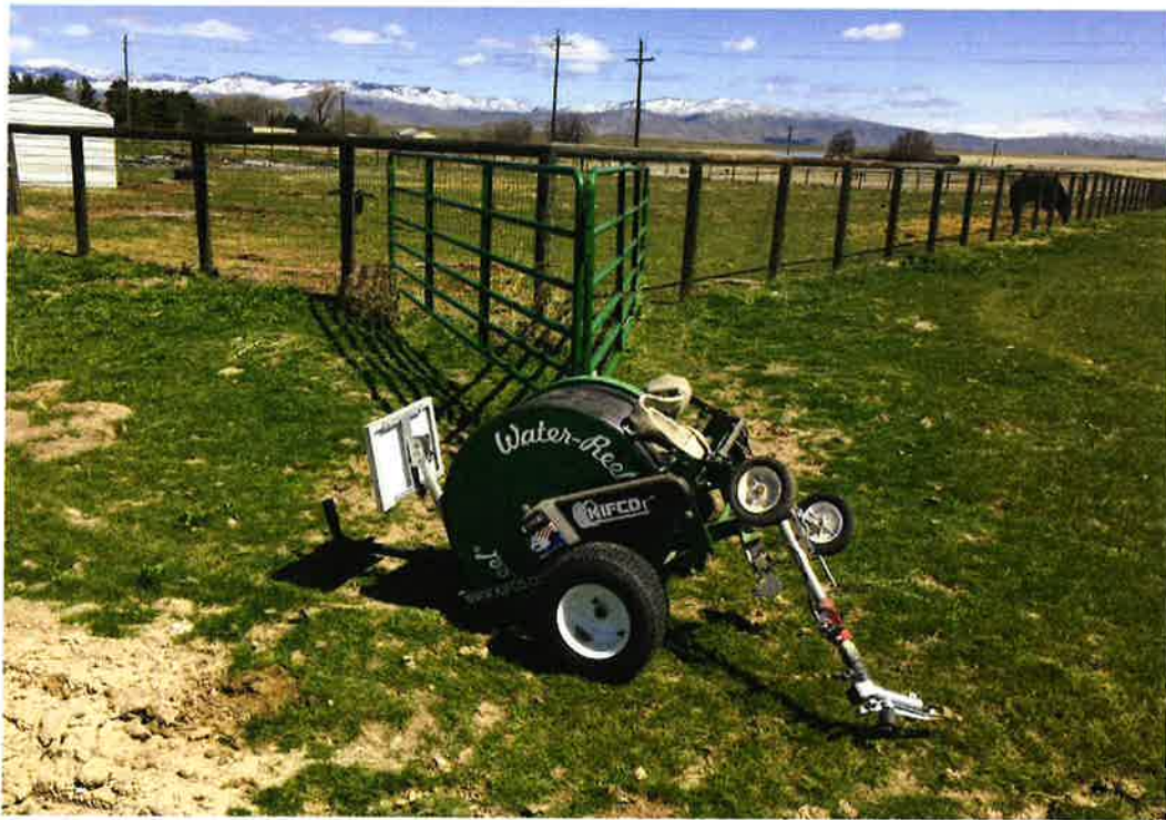
Hose-reel sprinkler at north tap
