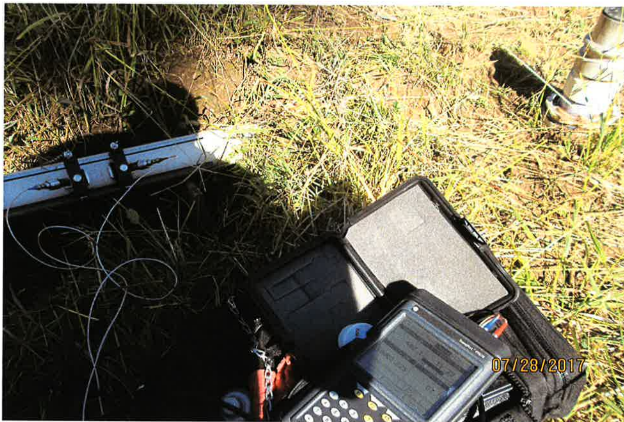
Performed flow measurement to see what well could produce and was equal to 445 gpm.
