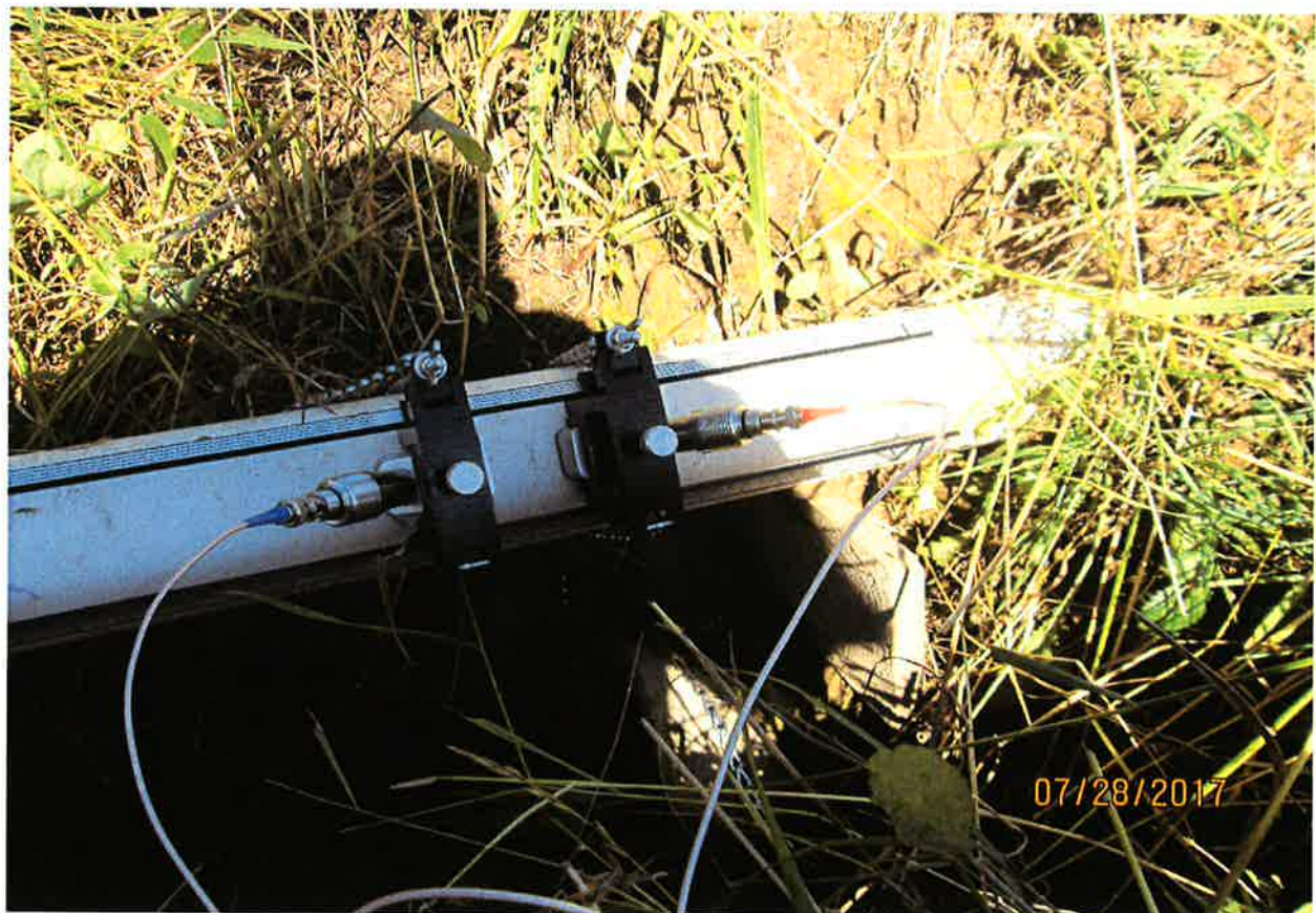
Flow measurement performed using GE Panametric Meter.
