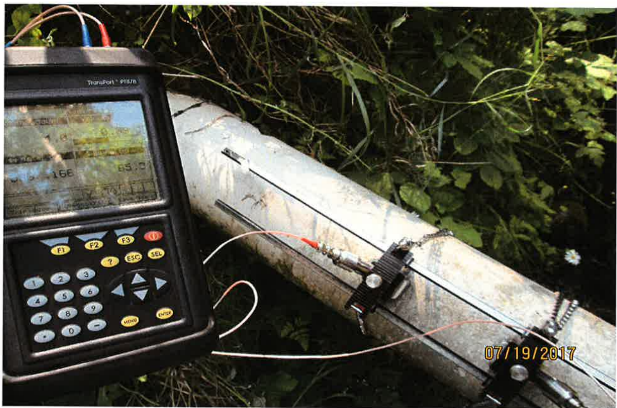
Flow measurement set up and meter running.
