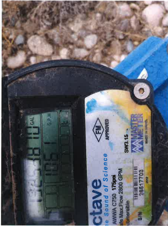
Figure 5 Octave flow meter used to measure flow during the field exam.
