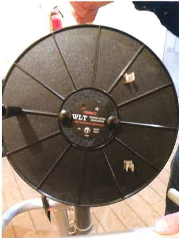
Figure 3 The e-tape used by the owner to measure water levels monthly
