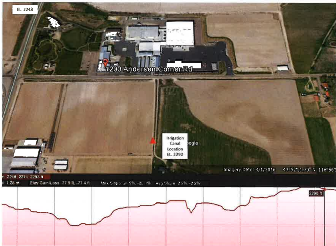
FIGURE 8: NUNHEMS AND FARMERS' COOPERATIVE SEBREE EXTENSION CANAL CONTROL STRUCTURE ELEVATION PROFILE
