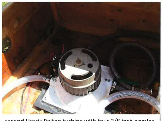
second Harris Pelton turbine with four 3/8 inch nozzles
