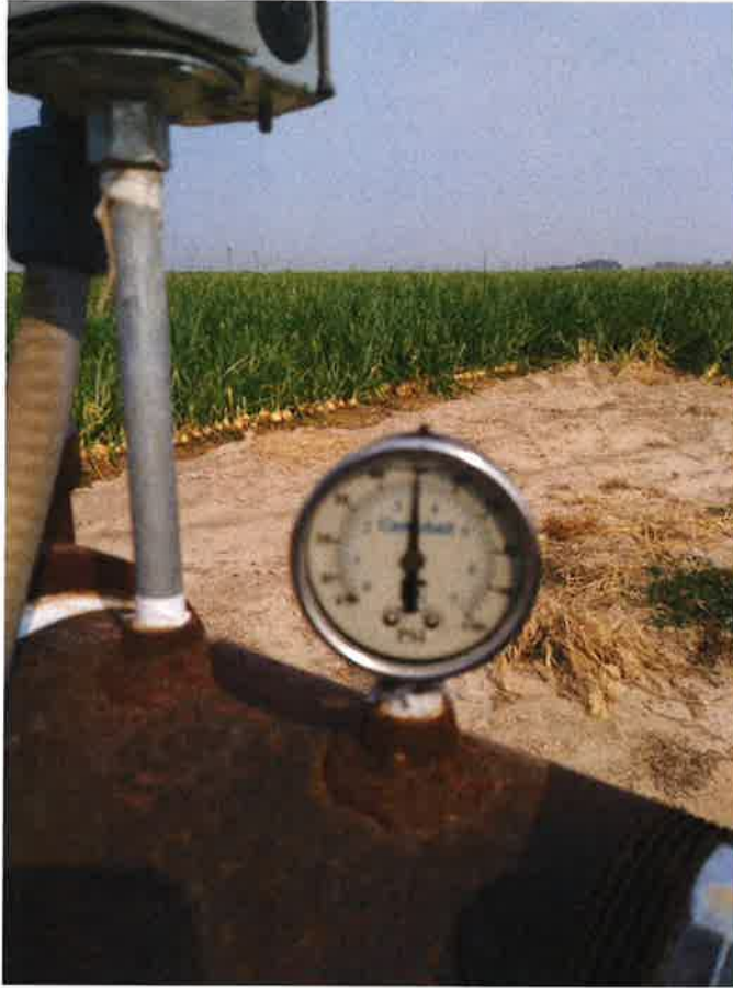
Figure 3. The operating pressure at the well head during the exam was 50 psi.
