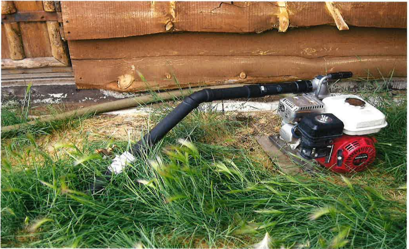
Pump and Hose with Fish Screen
