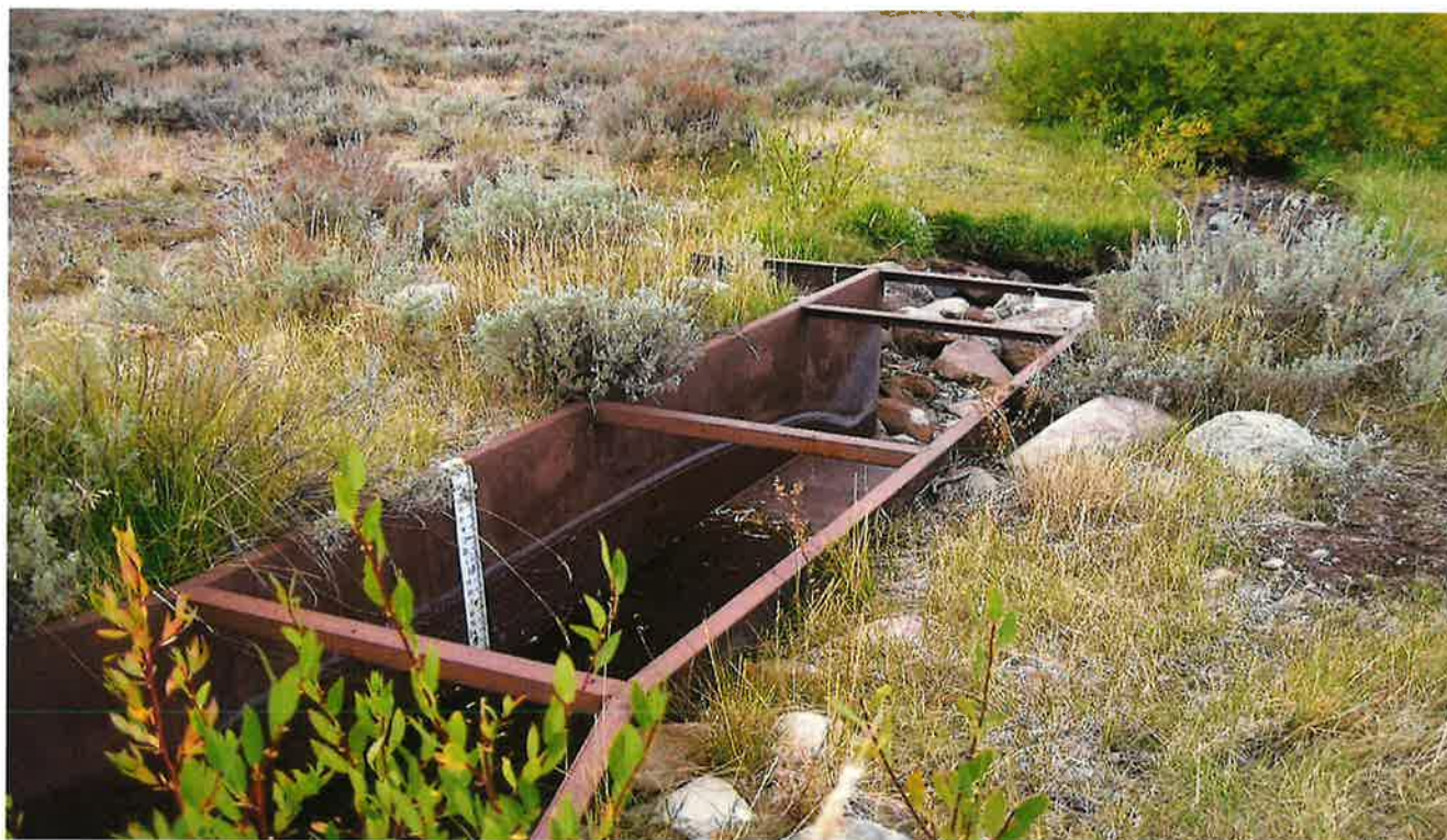
Ramp Flume Measuring Device and staff gage
