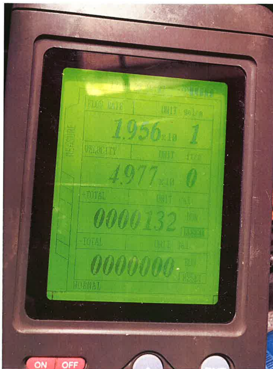
Figure 7: Portable ultra-sonic meter readout; maximum discharge associated with domestic use in the residence.
