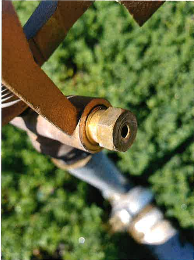
Figure 3. 7/64" nozzles on each sprinkler head on wheel lines.
