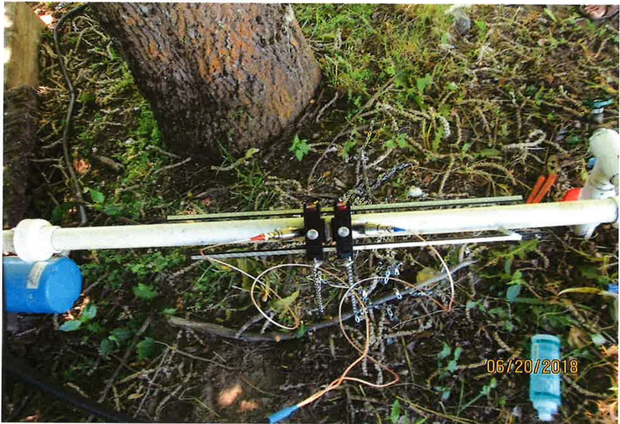
GE Panemetric flow meter used for measurement.
