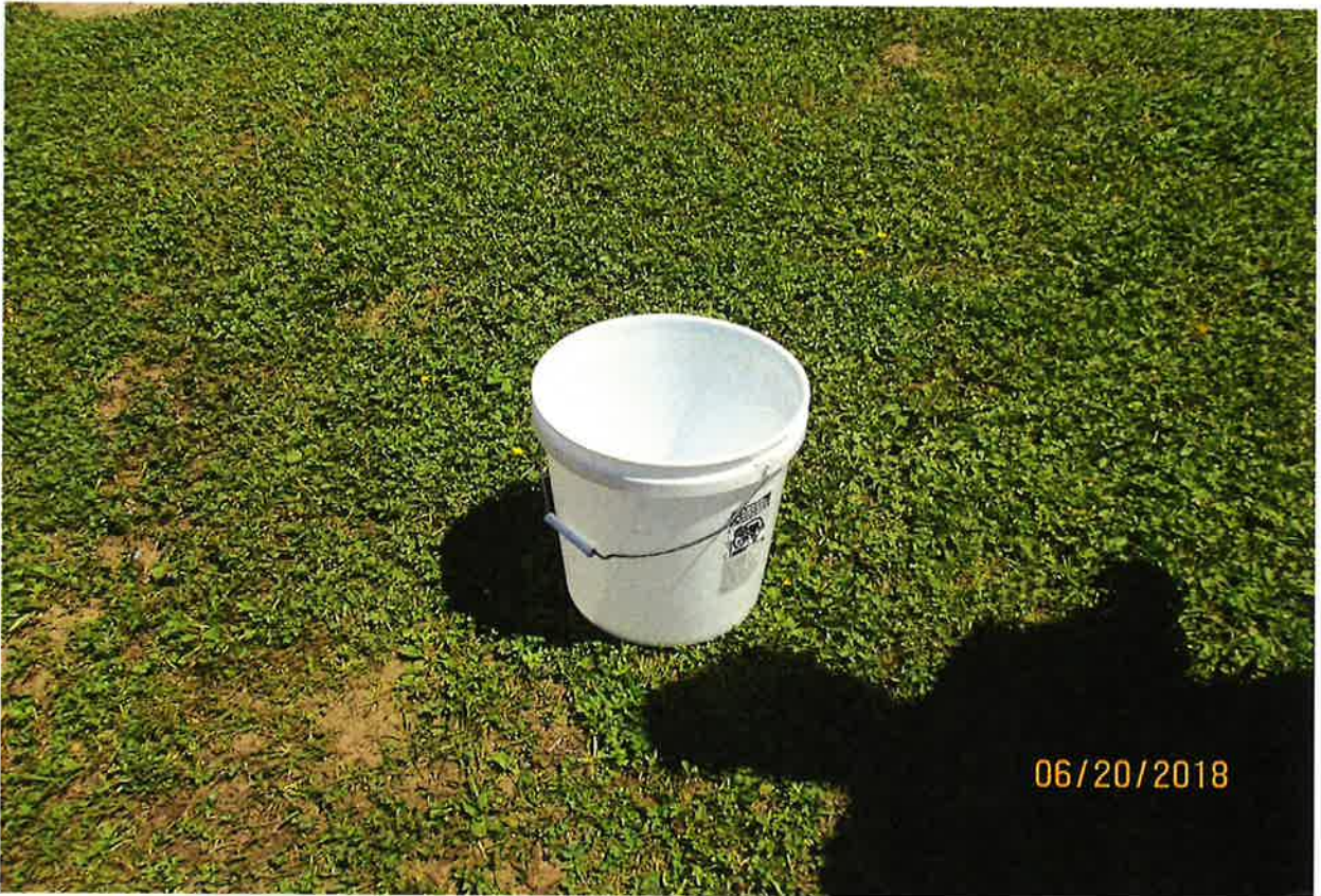
5 gallon bucket test performed in 9 seconds which is equal to 33 gpm or 0.07 cfs.
