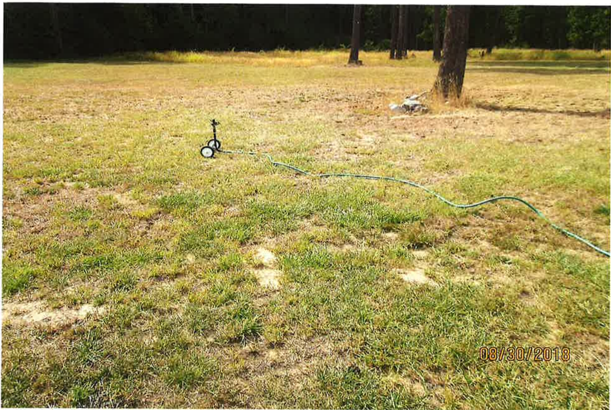
Irrigation sprinkler and hose used for 5 gallon bucket test in 34 seconds or 8.8 gpm or 0.02 cfs.
