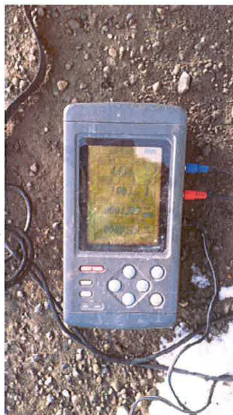
Flow meter readout for condition #6 in the 4" line
