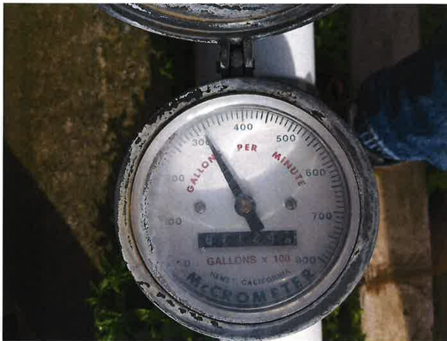
McCrometer propeller-type flow meter showing a diversion rate of roughly 315 gpm between the two wells.
