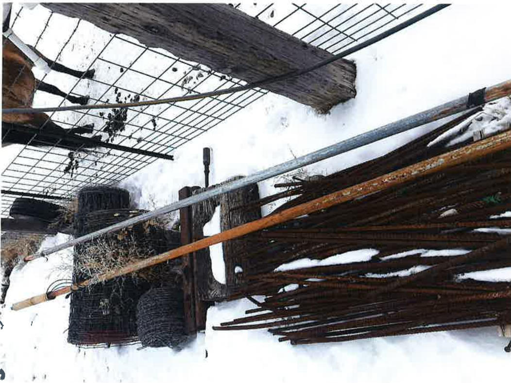
Figure 8. Pump and riser pipe recently removed from Schvaneveldt well.
