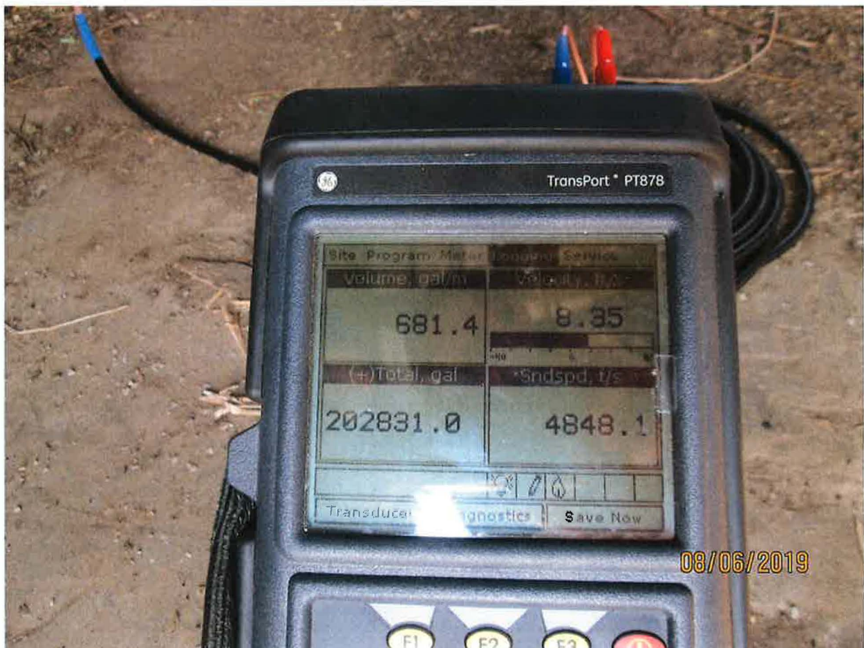
Flow measurement performed using GE Panametric Meter which was equal to 682.7 gpm or 1.52 cfs.
