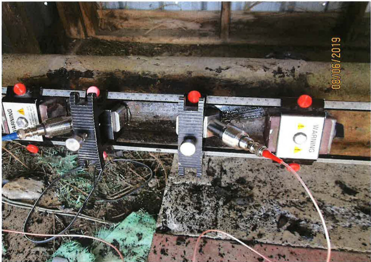
Flow measurement performed using GE Panametric Meter which was equal to 682.7 gpm or 1.52 cfs.
