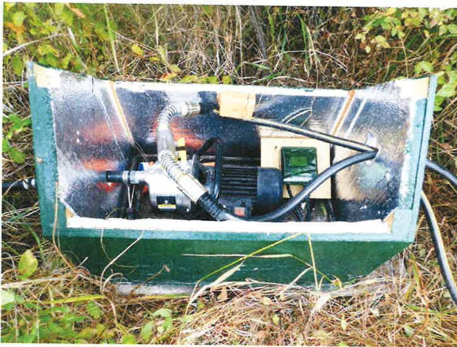
Pump House holding 1 hp Sprinkler Pump with timer drawing water from the Middlefork of the Payette. Distributes water via two hose pipes to above ground sprinklers per original application.
