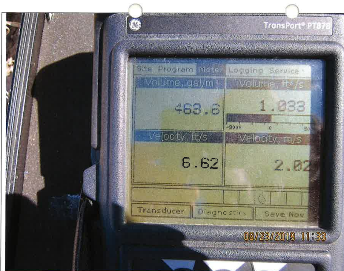
Figure 3. Panametrics flow meter reading a rate of 463.6 gpm or 1.03 cfs discharge.
