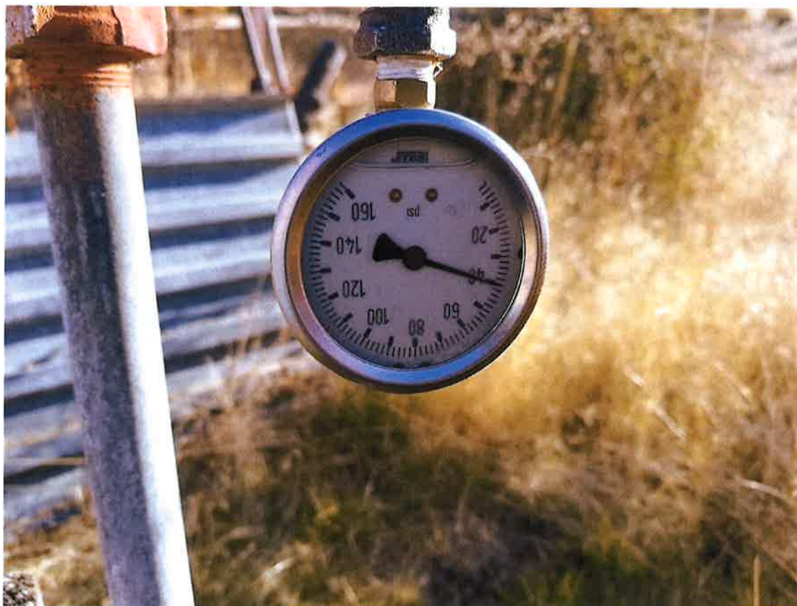
Looking at irrigation spigot #1 closest to house (1 of 4 spigots). Test yielded 40 psi.
