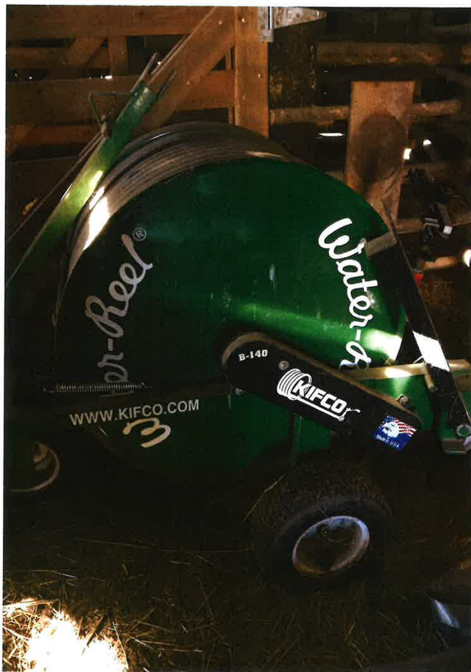
Portable irrigation line, Trailer and sprinkler. Hooks to pump.
