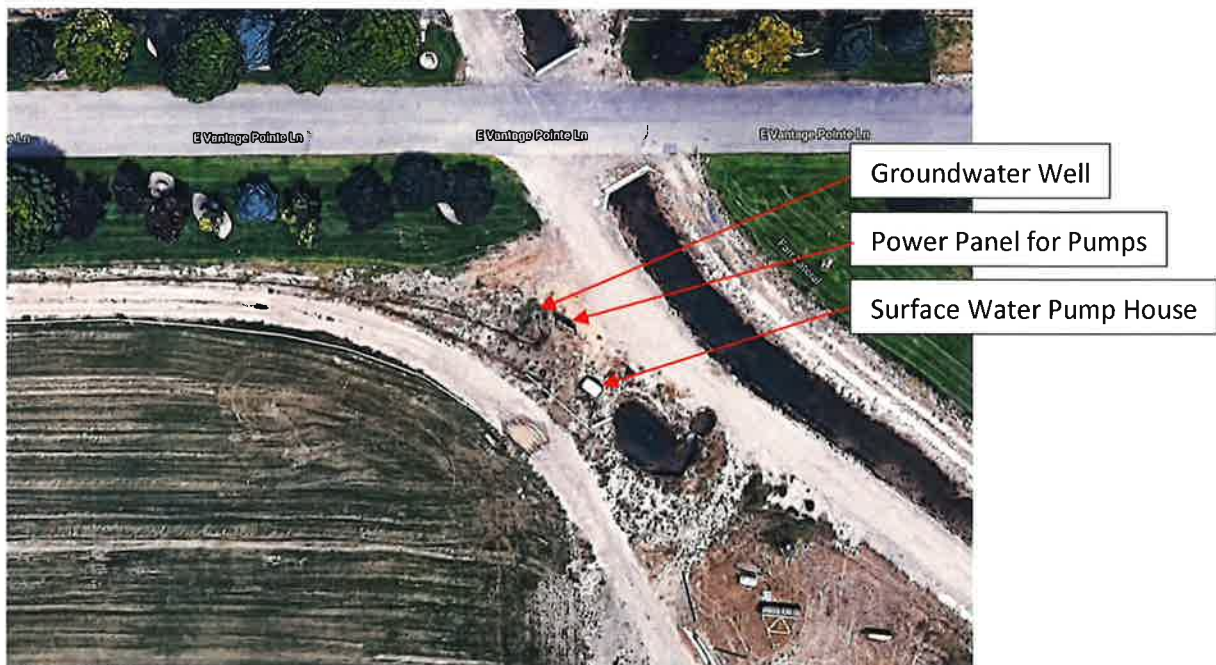
Aerial Photo from Google Maps showing the location of the groundwater well and surface water holding pond, Farr Lateral, and location of surface water pump.
