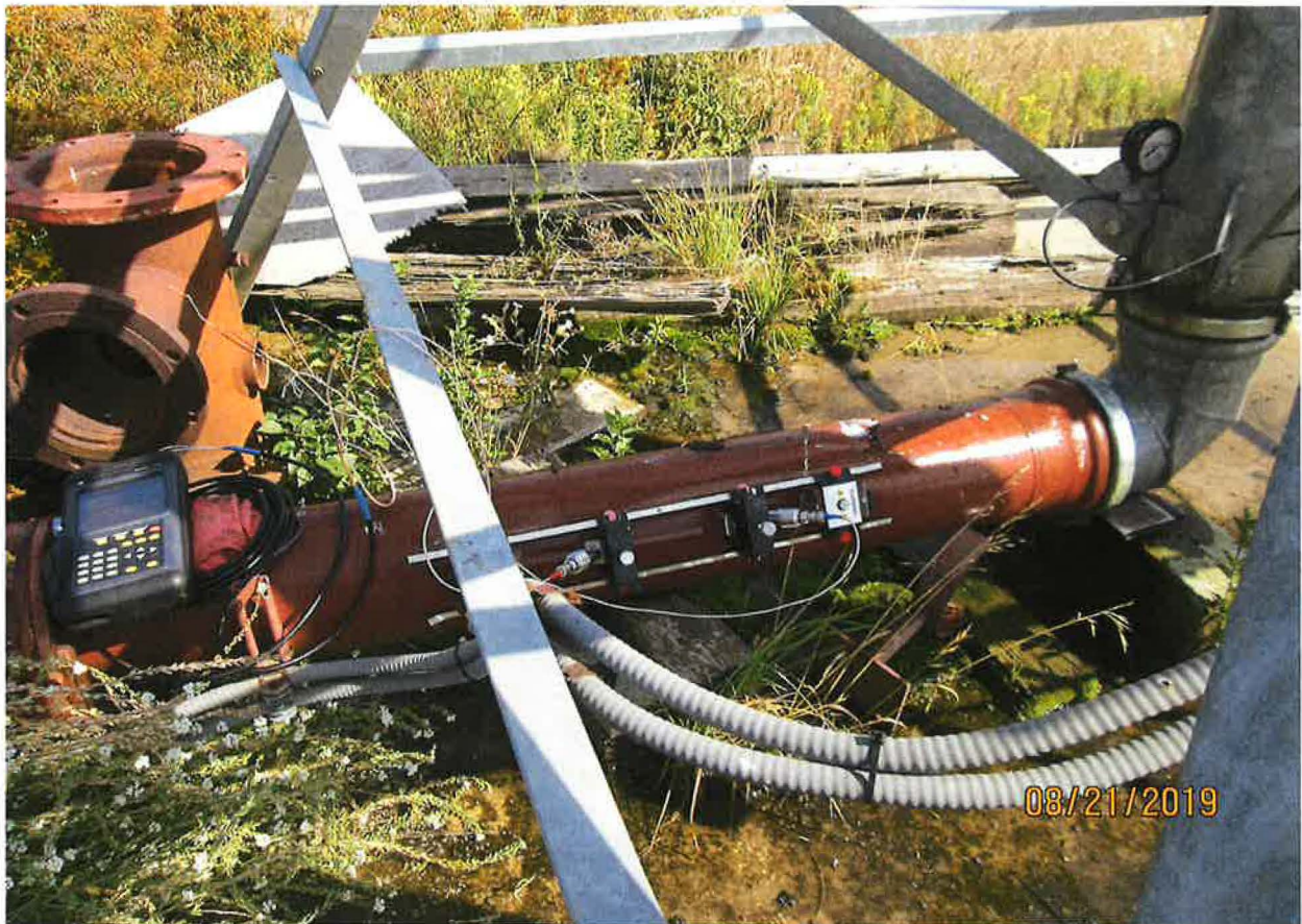
1 st flow measurement performed using GE Panemetric.
