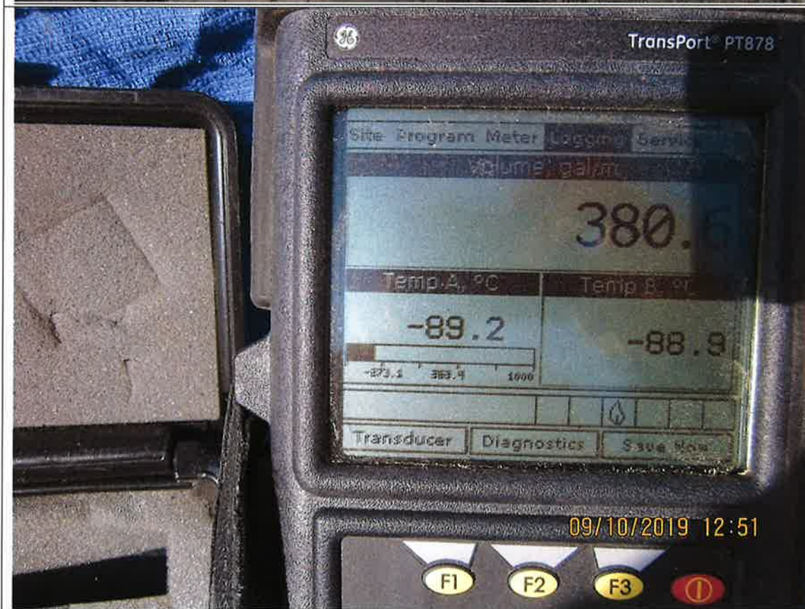
Figure 10. Panametric flow meter measurement was 380.6 gpm or 0.85 cfs.
