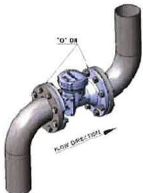
Zero (0) pipe diameters permitted before & after elbows (90°)
