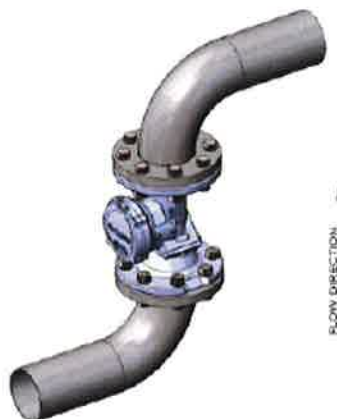
Zero (0) pipe diameters before and after elbows (90°) in vertical installations
