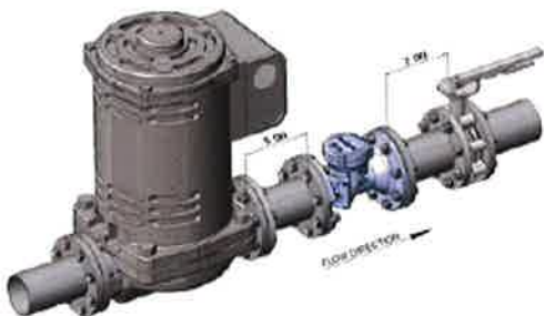
Minimum of five (5) pipe diameters after pump discharge.
