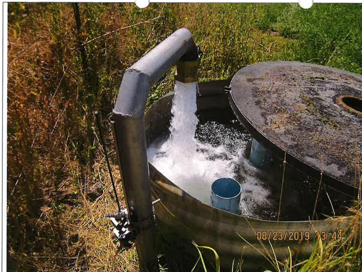
Figure 5. Bubbler receiving well water from source pipe with Panametrics transducers attached.
