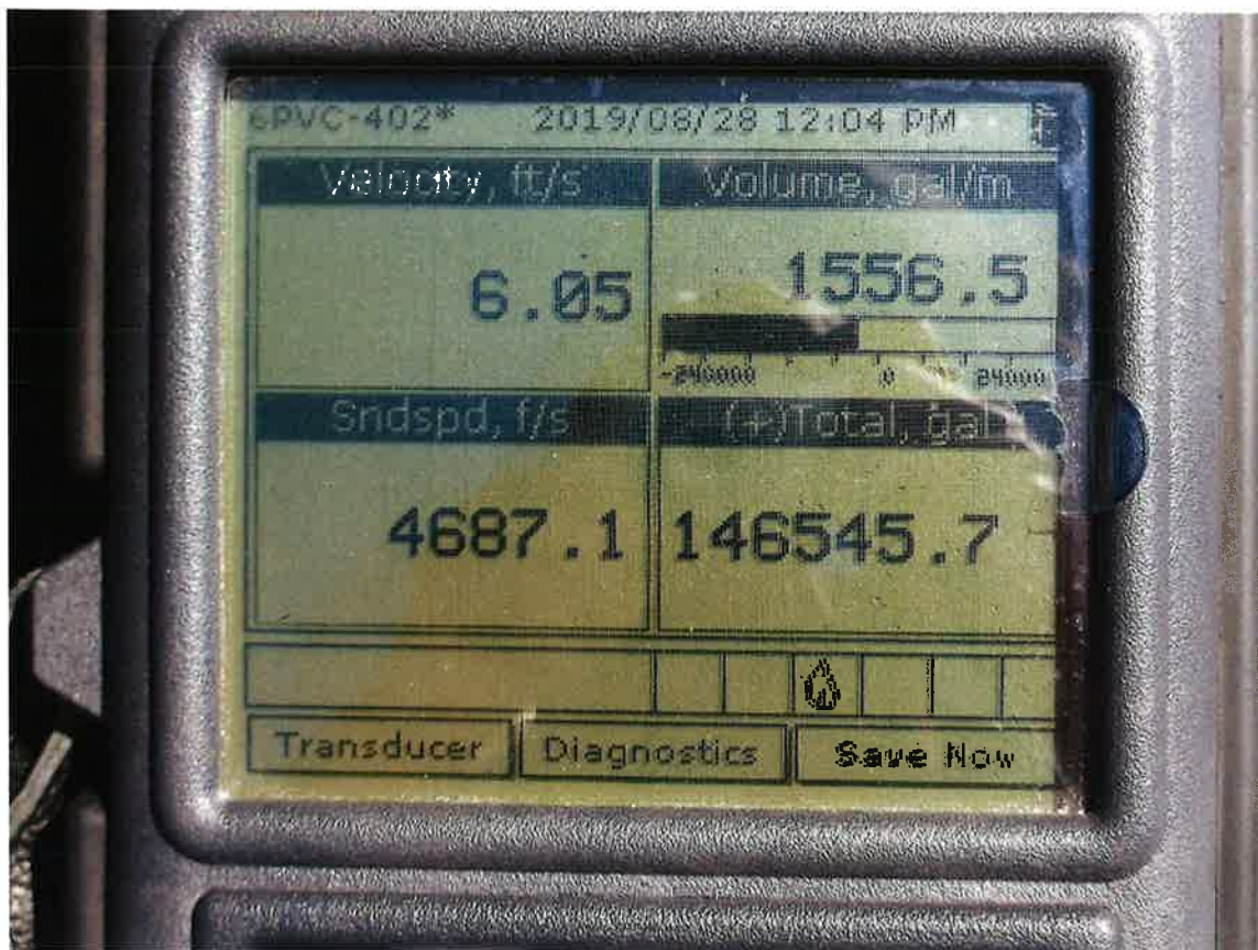
IDWR portable flowmeter reading at lower (south) well.
