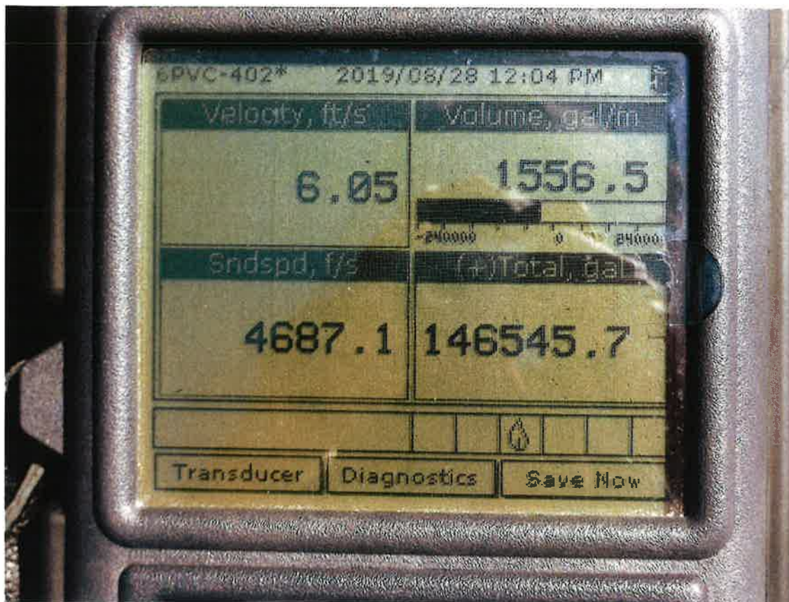
IDWR portable flowmeter reading at lower (south) well.
